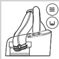
*Note: When the fluid level drops below the minimum level, the cleaning symbol and the 'fluid low' symbol start to flash and the shaver holder returns to its starting position.*
