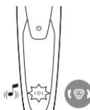
The replacement reminder indicates that the shaving heads need to be replaced. The shaving unit symbol lights up continuously, the arrows flash white and you hear a beep when you switch off the shaver.
