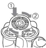
Note: Hold the shaving head holder in your hand when you reinser the shaving heads and reattach the retaining rings. Do not place the shaving head holder on a surface when you do this, as this may cause damage.
