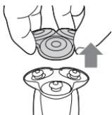
**3** Switch off the shaver. Pull the shaving head holder off the bottom part of the shaving unit.
