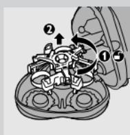
**1** Open the shaving unit, turn the lock anticlockwise (1) and remove the retaining frame (2).
