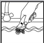
**3** You can also immerse the Razor Head Assembly in hot water for at least 30 seconds.
