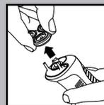
**2** Remove Razor Head Assembly from razor by pulling Razor Head Assembly straight up from razor.
