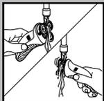
**2** Rinse Razor Head Assembly under hot water by letting the water run in and around all the openings for at least 30 seconds.
