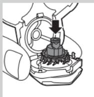
**7** After cleaning, place the cutter back into the shaving guard with the cutter legs pointing downwards.
