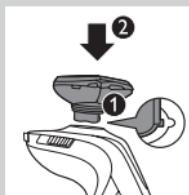
**10** Insert the lug of the shaving unit into the slot in the top of the shaver (1). Then press the shaving unit downwards (2) to attach it to the shaver ('click').
