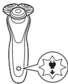
The 'unplug for use' reminder flashes to remind you to disconnect the shaver from the wall socket before you can switch it on.
