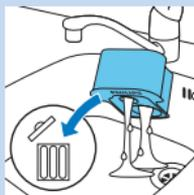
**2** Take the empty cleaning cartridge from the SmartClean system and pour any remaining cleaning fluid out of the cleaning cartridge.
