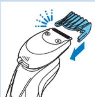
**1** Slide the comb straight into the guiding grooves on both sides of the beard styler attachment ('click').
