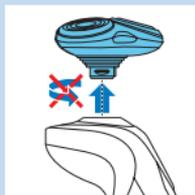
**2** Insert the lug of the trimmer attachment into the slot in the top of the shaver. Then press down the trimmer attachment to attach it to the appliance ('click').
