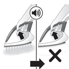
Besides that, a second defense step to protect the steam generator from scale is integrated: the steam function gets disabled if descaling is not done. After descaling is done, the steam function will be restored. This takes place regardless of the type of water used.
