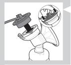
For battery operation (SCF332 only), turn the bottom of the motor unit in the direction indicated by the marks on the bottom (1) and remove it (2). Insert four new 1.5V AA batteries (or 1.2V, if rechargeable) into the battery housing. Reattach the bottom to the motor unit.
