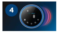
The color ring provides an additional visual cue ranging from blue (good) to red (poor) to present the indoor air quality.
