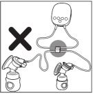
9 Connect the power adapter to the pump motor, and then insert the power plug to the power socket.
