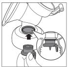
2 Put the bottle onto the pump body and turn it anticlockwise to fix it. Do not over-tighten when assembling the bottle to the pump body.
