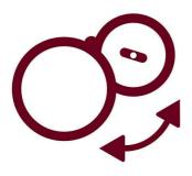
The filter holder is opened by swinging it to the side, which makes the filling of coffee easy. The filter holder is also detachable, for easy cleaning.
