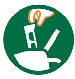
The removable micro-mesh filter on the spout restrains all scale particles with size > 200 micron and ensures that the water you put into your cup is clean.
