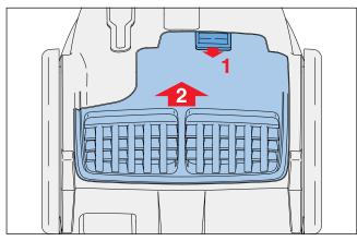
• Remove the dustcover assy (7) using a screwdriver (see picture).
