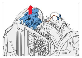
• To remove the Motor housing: Remove the 4 screws (**E**), for 2 of the screws an extra long screwdriver is needed. (see picture)
