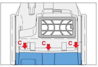
• Lift the Top housing by using a screwdriver on the backside, place it between Lower housing and Top housing.
