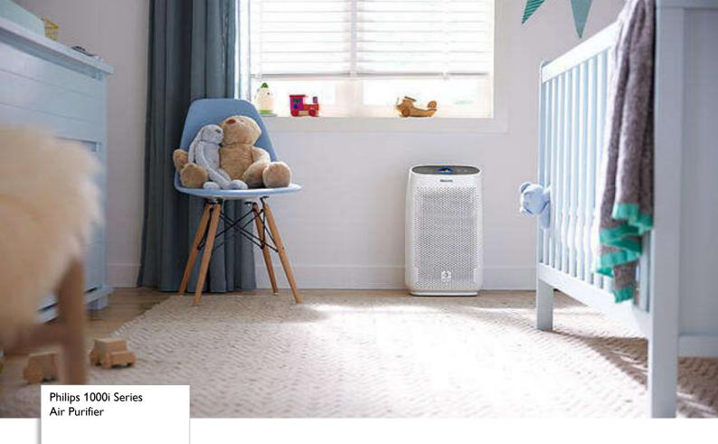
Purifies rooms up to 63 m<sup>2</sup> 270 m<sup>3</sup>/h clean air rate (CADR) HEPA & Active Carbon filter
