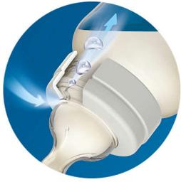
Our clinically proven Airflex venting system is designed to reduce gas and colic. As your baby feeds, the valve integrated into the nipple flexes to allow air into the bottle to prevent vacuum build up and vents it towards the back of the bottle. It keeps air in the bottle and away from baby's tummy to help reduce gas, spit-up and burping.
