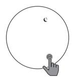
**Auto mode ( ( ):** In Auto mode, the dual-sensor sense the air quality in real-time and the appliance automatically adjusts the fan speed in accordance with the ambient air quality, the control panel can automatically adjust display screen brightness according to the ambient light.
