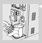
5 When the dispensing has finished, empty the container and place it under the water dispenser.
