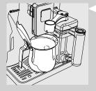
15 Empty the container and place it back under the coffee dispensing spout. Open the milk dispenser by turning it clockwise.
