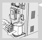
6 At the end, remove the container with the desired quantity of water.
