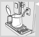
17 Place a container under the dispensing spout to catch the small amount of water which will be dispensed.
