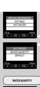
2 Select HOT WATER by pressing the "√" or "∧" scrolling button. Press "OK" to confirm.
