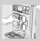
The height of the dispensing spout can be adjusted to better fit the dimensions of the cups that you wish to use.
