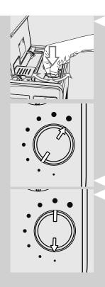
2 Press and turn the grinder adjustment knob one notch at a time. You will taste the difference after brewing 2-3 cups of espresso.
