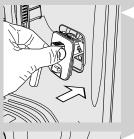
1 Slightly tilt the water dispenser and then insert it in into the guides in the machine.
