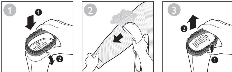
**EN** The brush attachment improves steam penetration into thick and heavy fabrics for faster results. This is meant to be used with steam. Hold the steam trigger and brush slowly with the bristles touching the garment.
