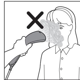
**EN** Do not use your bare hand as a supporting surface when you steam. Pull the sides of the garment to stretch it. Do not place the steamer head on the power cord after use.
