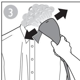
**EN** Hold the trigger and move the steamer horizontally along the collar.
