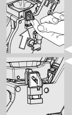
13 Make sure that the hook which locks the brew group is in the correct position. If it is still in the downward position push it upward until it locks correctly into place.
