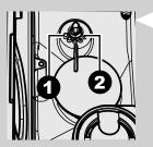
3 The reference marks inside the coffee bean hopper indicate the grind setting. There are 5 different grind settings to choose from, from position 1 (●) for coarse grind - milder taste to position 2 (•) for fine grind - stronger taste. If coffee is watery or is brewed slowly, change the coffee grinder settings.
