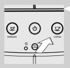
Press the "" button. The machine starts brewing coffee. Wait until brewing has been completed and empty the container.
