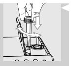
While the machine grinds coffee, press and turn the grinder adjustment knob placed inside the coffee bean hopper one notch at a time. Use the special coffee grinder adjustment key supplied. You will taste the difference after brewing 2-3 cups of coffee.
