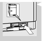
12 Switch the power button to "I". The "(1)" button flashes.
