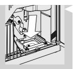
14 Insert the coffee residues drawer in its seat and ensure that it is correctly in place.
