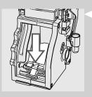
III Gently pull down the lever until it is in contact with the brew group base and the two reference marks on the side of the brew group match.
