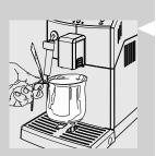
When the warm-up phase has been completed, the machine automatically performs a rinse/self-cleaning cycle of the internal circuits with fresh water. This takes less than a minute.
