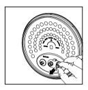
To assemble the floater, put the thin end of the floater into the hole on the lid (fig.(1)), and assemble the rubber ring around the floater (fig.(2)).
