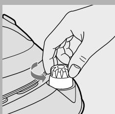
Do not open the cap when the appliance is hot and the steam tank is still under pressure.
