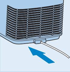
**2** To store excess cord, push it into the storage compartment at the back of the appliance.
