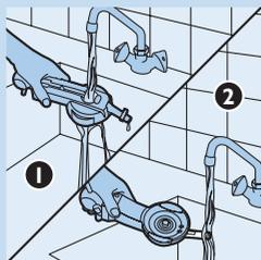
**3** Then turn the tap unit upside down and rinse the keg connection in the bottom of the tap unit.
