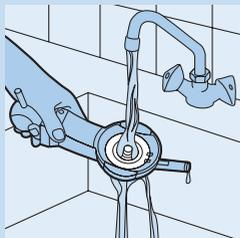
**4** Check if the tube release button works properly. When you press the blue tube release button, the two clamps in the opening have to move.
