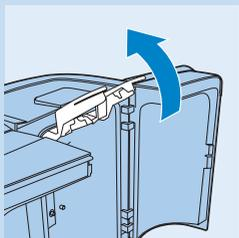
**2** Lift the two blue locking levers completely.
