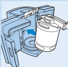
**3** Tilt the keg with the assembled tap unit slightly forward and put it into the appliance.
