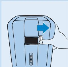
**1** Slide the release button to the right to open the doors.
