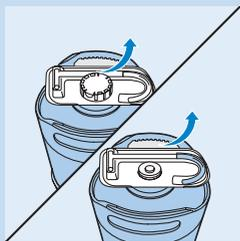
**2** If present, remove the tube connector and the tube from the tap unit. Hold the tap unit under a running tap and rinse the tube-connection hole (1) and the connection to the body of the appliance (2). If necessary, use some washing-up liquid.
