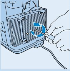
**6** Undo the screws with a screwdriver.
