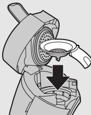
**5** Put the 1-cup pod holder or the 2-cup pod holder in the machine without pod(s).
