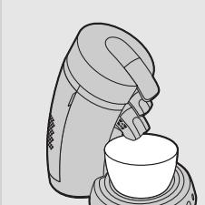
**8** Put a bowl (with a capacity of at least 1500 ml) under the spout openings to collect the water.
