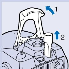
The crevice nozzle can be used either for cleaning narrow corners or hard-to-reach places.
