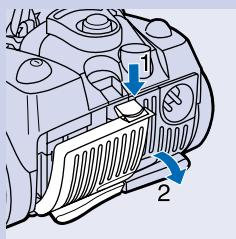
Some appliances are equipped with an ACF-S Combi Filter. This filter not only removes household dust, but also harmful microscopic vermin. It also absorbs 80% of all unpleasant smells.
