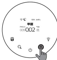
**Sleep mode (☾):** The air purifier operates quietly at a low speed. After 3 seconds, the screen lights off.
