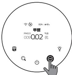
**Auto mode (A):** The air purifier automatically adjusts the fan speed in accordance with the ambient air quality.
