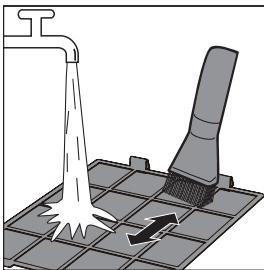
**5** Allow the pre-filter to air dry thoroughly before placing back in the air purifier.
