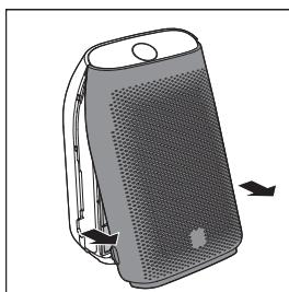
2 Press the two clips down (1) and pull the pre-filter towards you (2).
