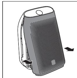
3 Press the two clips down (1) and pull the pre-filter towards you (2).
