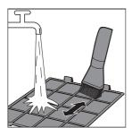
5 Allow the pre-filter to air dry thoroughly before placing back in the air purifier.
