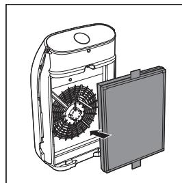
6 Attach the pre-filter back into the air purifier.
