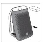
2 Press the two clips down (1) and pull the pre-filter towards you (2).
