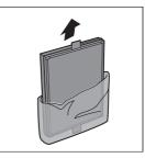
4 Place the new filter into the air purifier.
