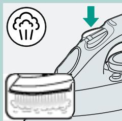
A powerful 'shot' of steam helps remove stubborn creases. The shot-of-steam function can only be used at temperature settings between ●● and MAX.
