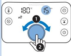
**9 To change the cooking time, turn the QuickControl dial to the desired setting.**
