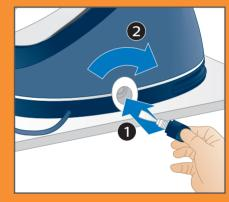
When no more water comes out, reinsert the EASY DE-CALC knob and turn it clockwise to tighten it.
