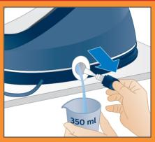
Remove the EASY DE-CALC knob and let the water with scale particles flow into the cup.
