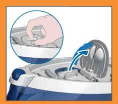
Remove the iron from the iron platform and open the ANTI-CALC cartridge compartment.
