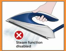
The steam function will be disabled automatically if the ANTI-CALC cartridge is not replaced.
