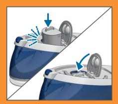
**Press down** the ANTI-CALC cartridge in the compartment until it **locks into place** and close the lid.
