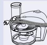
► Wrap the mains cord around the bowl. Use the suction cap to keep the cord in place.
