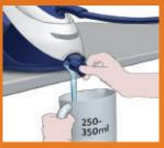
**Remove the EASY** DE-CALC knob and let the water with scale particles flow into the container. When empty, fasten the knob turning it clockwise.
