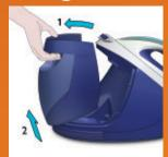
Remove the water tank from the base.
