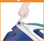
Press the carry lock release button to unlock the iron from the base.
