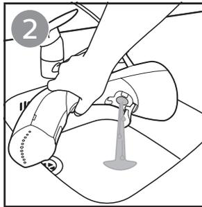
EN Wipe any deposits off the steamer head with a damp cloth and a non-abrasive liquid cleaning agent.
