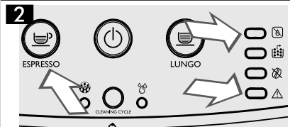
"ESPRESSO" steady on and "LUNGO" and "CLEANING CYCLE" flashing
