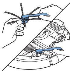
Tip: If bristles of the side brushes are crooked or bent, soak the side brushes in warm water for a while. If this does not restore the bristles to their proper shape, replace the side brushes (see 'Replacing the side brushes').
