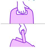
This vacuum cleaner has not one, but two carrying handles. When it is on its wheels, there is a handle on top which enables you to easily move the cleaner around with very little bending. The second handle on the front side of the appliance enables you to comfortably carry it around in an upright position.
