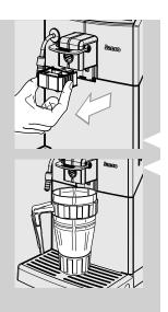
Remove the lower part of the dispensing spout to allow a tumbler to be used.
