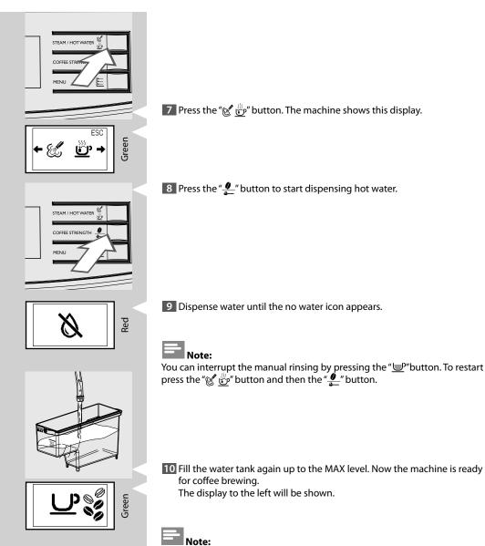
When the machine has not been operated for at least two weeks, it will automatically perform a start-up rinse/self-cleaning cycle. Following this, you need to initiate a manual rinse cycle as described above.
