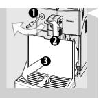
**4** Insert the coffee grounds drawer back into the drip tray and this into the machine.
