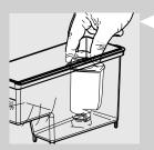
4 Put the "INTENZA+" water filter into the empty water tank. Press it down until it cannot move any further.
