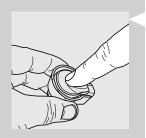
**23** Attach the lid by pressing in the middle, and ensure that it is firmly in place.
