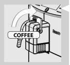
2 Push the lever upwards to select the "COFFEE" function.
