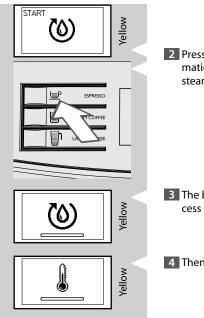
Press the "" button to start the cycle. The machine starts the automatic priming of the circuit by dispensing some water through the steam wand.
