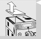
4 Lift the water tank using the handle.
