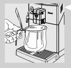
Place a container under the dispensing spout to catch the small amount of water which will be dispensed.
