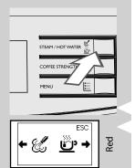
**3** Press the "😢 📴" button. The machine shows this display.
