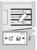
**2** Press the "🗭 📅" button. The machine shows this display.
