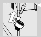
3 Insert the Automatic Milk Frother until it locks in place in the steam wand seat.
