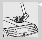
3 Lift the pre-ground coffee compartment lid and add one scoop of preground coffee to the compartment. Use only the measuring scoop supplied with the machine. Then close the pre-ground coffee compartment lid.
