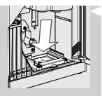
11 Insert the coffee residues drawer in its seat and ensure that it is correctly in place.
