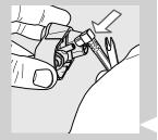
2 Insert the suction tube into the Automatic Milk Frother.
