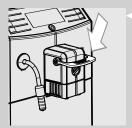
This selection must be made prior to brewing a beverage by simply moving manually the lever positioned on the dispensing spout.
