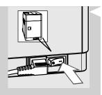
2 Switch the power button to "I" to turn on the machine. The "()" button flashes.
