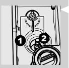
2 The reference marks inside the coffee bean hopper indicate the grind setting. There are 5 different grind settings to choose from position 1 for coarse grind - milder taste to position 2 for fine grind - stronger taste
