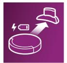
When the battery of the Philips robot vacuumcleaner is almost empty, it will automatically go to the docking station to charge itself, so it will get ready for its next cleaning session.
