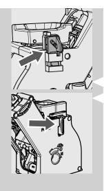
10 Make sure the hook to lock the brew group is in the correct position by firmly pressing the "PUSH" button until it locks into place. Check if the hook is at the top end position. If it is not, please try again.
