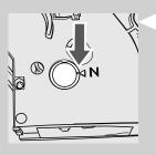
9 Gently pull down the lever until it is in contact with the brew group base and the two reference signs on the side of the brew group match.
