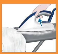
Press and hold the steam trigger for steam during ironing.
