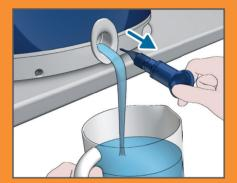
Remove the EASY DE-CALC knob and let the water with scale particles flow into the cup.
