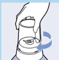
**4** Turn the assembled mill upside down and screw it onto the motor unit in the direction of the arrow.
