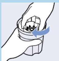
**3** Screw the blade unit onto the beaker.
