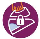
Your steam generator iron includes a safe carry lock, which securely fastens your iron to its base without the risk of it slipping or someone touching the hot soleplate. It ensures safe and easy transportation around the house, to and from storage.
