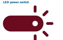
The red light on the switch button illuminates when the coffee maker is switched on.
