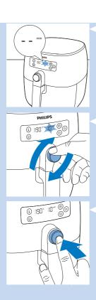
9 After the temperature is confirmed, the time indication "--"starts blinking.
