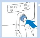
→ To confirm the cooking temperature or time, push the QuickControl dial.
