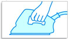
The ergonomic design of the iron facilitates comfortable ironing by putting less strain on the wrist. The upwardly sloping handle ensures a natural position reducing strain during ironing. The iron design also prevents the repetitive movements caused by placing an iron on its heel. The iron is light (1.2 kg) for an easy and comfortable ironing experience.
