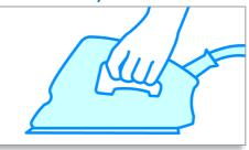
For your safety, the automatic safety shut-off switches the ironing system off when it is left unattended. The ironing system can be reactivated by pressing any button.
