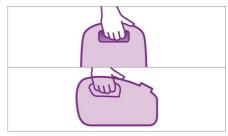
This vacuum cleaner has not one, but two carrying handles. When it is on its wheels, there is a handle on top which enables you to easily move the cleaner around with very little bending. The second handle on the front side of the appliance enables you to comfortably carry it around in an upright position.
