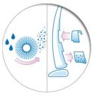
Separate clean and dirty water tanks ensure that you always mop with clean water, so you avoid spreading the dirt around.
