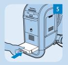
Slide the rinse tray back into the appliance. The appliance stops beeping and the red light goes out.
