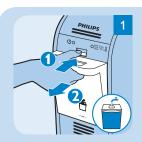
Put the mains plug **(1)** in an earthed wall socket. The power-on light goes on. **Fill the water tank.**
