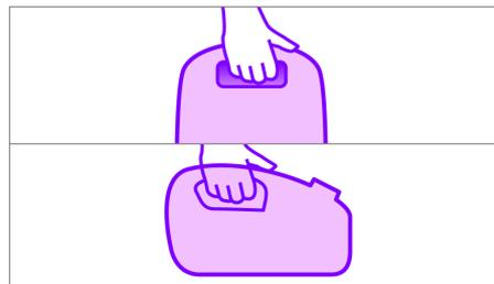
This vacuum cleaner has not one, but two carrying handles. When it is on its wheels, there is a handle on top which enables you to easily move the cleaner around with very little bending. The second handle on the front side of the appliance enables you to comfortably carry it around in an upright position.
