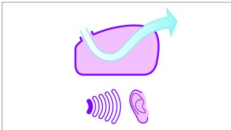
The air channel has been finetuned to make sure the air slides a smooth way out that minimizes noise creation. Additionally a special motor suspension reduces vibrations.
